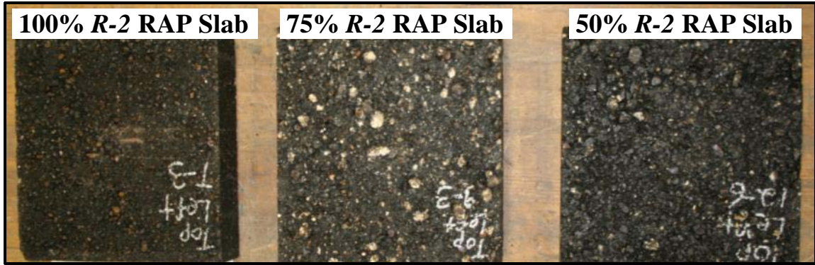
Figure 10.18 Laboratory Mixing Efficiency for High RAP Contents ( R-2 RAP Shown )
