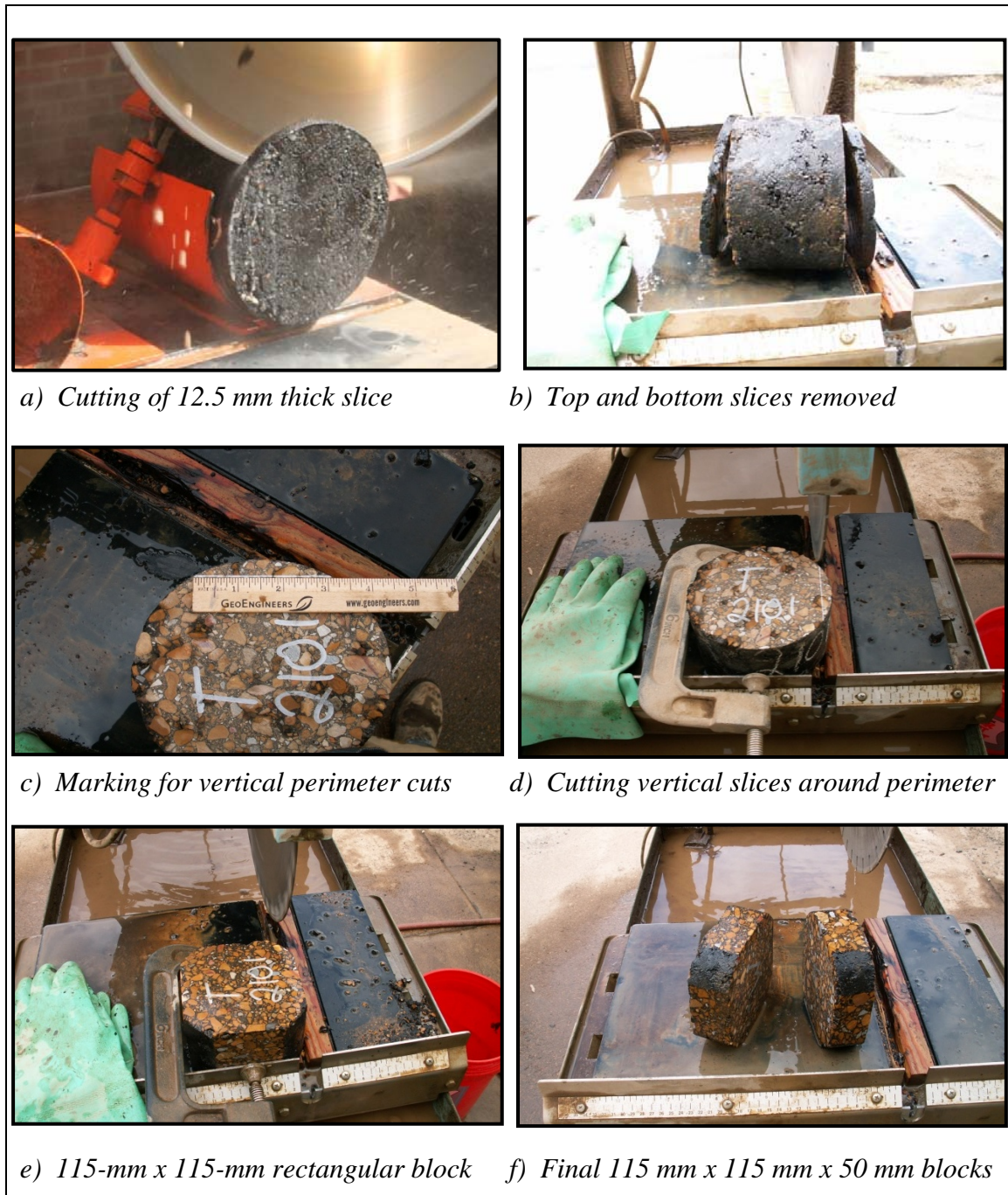
Figure 3.8 Step 1-Rectangular Block Preparation for BBR Specimen Production
