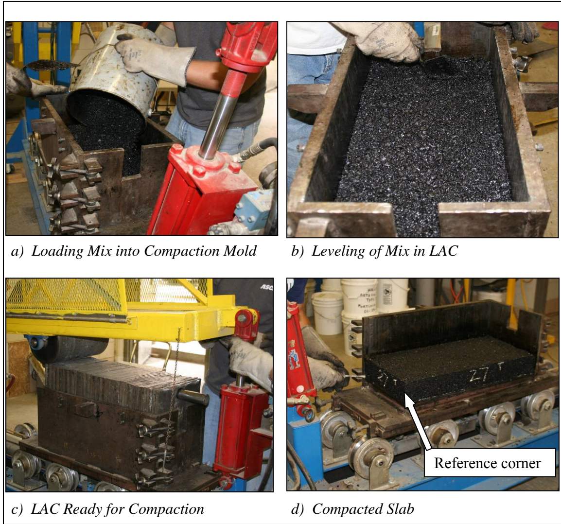
Figure 3.6 LAC Slab Compaction Process
